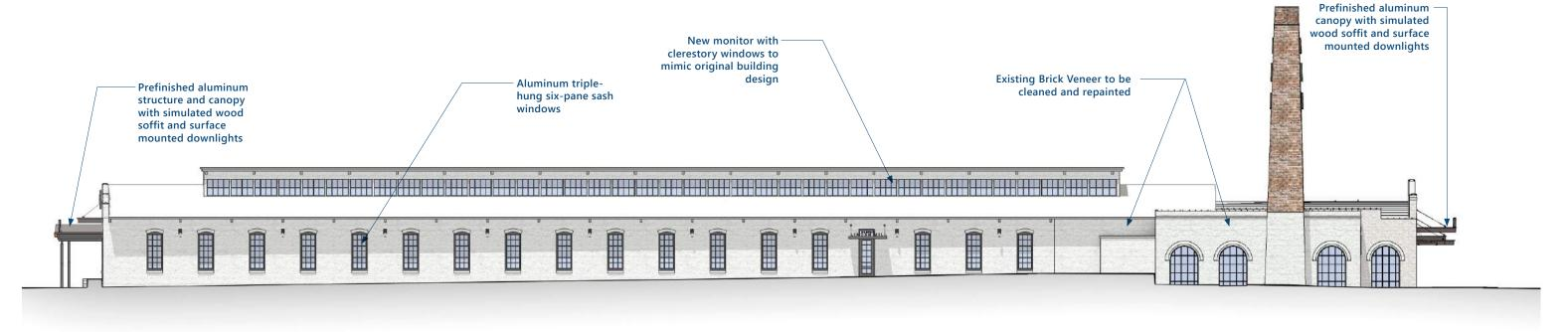
South Elevation (Facing Eden St.)
