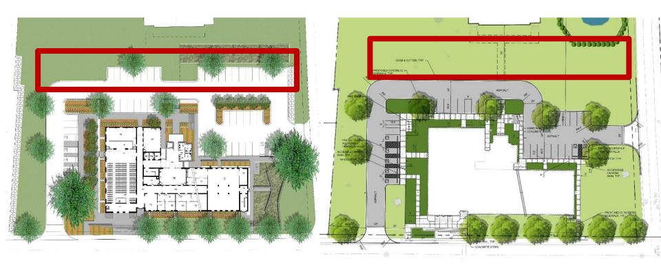
Parking spaces reduced, concrete walls removed, some stormwater modifications. Additional reductions possible.
