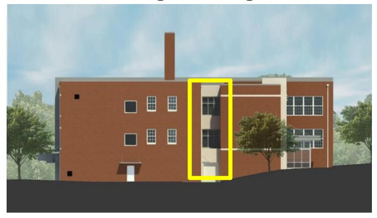
Addition connector changed to painted fiber cement board versus pre-cast concrete
