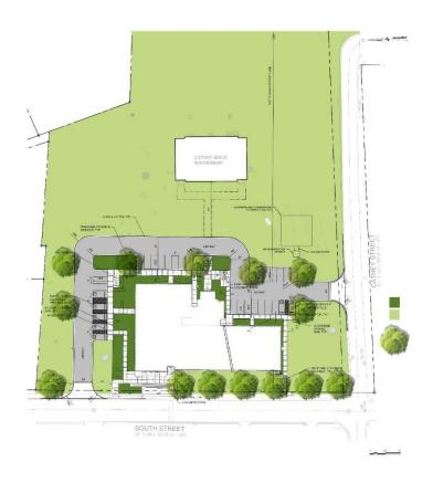
Above ground retention show on left, below ground on right
